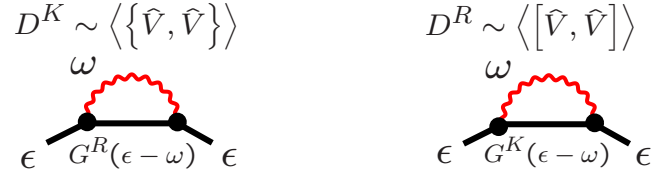
FIG. 4. (Color online) Contributions to the decoherence rate in a Keldysh-diagrammatic treatment. Left: Diagram involving both thermal and quantum fluctuations of the bath, but no Fermi distributions. This diagram is the same in a single-particle situation. Right: Diagram corresponding to the “backaction” term discussed in the equations of motion approach. It involves the fermionic Keldysh Green's function [that contains the Fermi distribution, G^K(\epsilon - \omega) \propto 1 - 2f(\epsilon - \omega) ] and the bath's retarded propagator (describing the response).
