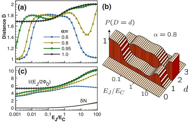
FIG. 3. (Color online) (a) Average many-body distance  $\bar{D}$  between the left- and right-going current states forming the ground state of a three-junction flux qubit at  $f=0.5$ , plotted as a function of  $E_J/E_C$ , for various asymmetry parameters  $\alpha$ . (b) Corresponding probability distribution for  $\alpha=0.8$ . (c) Magnitude  $I$  of the average current in the two current states, and average charge fluctuation  $\delta N$  in the ground state [symbols as in (a)].
