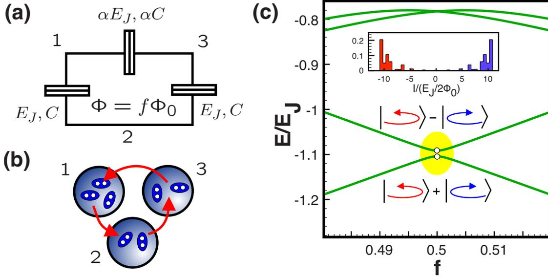
FIG. 2. (Color online) (a) Circuit diagram of the three-junction flux qubit. (b) Equivalent representation in the charge basis. (c) Energy-level diagram for  $E_J/E_C=20$  and  $\alpha=1$ , as a function of magnetic frustration. At  $f=0.5$ , the ground and first excited state are superpositions of left- and right-going current states,  $|\pm I\rangle$ , the states between which we calculate the “distance”  $D$ . The current distribution in the ground state is displayed in the inset.
