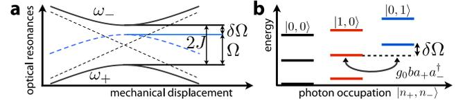
FIG. 2 (color online). (a) Optical resonances vs mechanical displacement. For  $\delta\Omega = 2J - \Omega \ll \Omega$ ,  $J$ , the regime of enhanced quantum nonlinearity is reached. (b) Energy level scheme of the double cavity optomechanical system. The most relevant second-order transition process is indicated.
