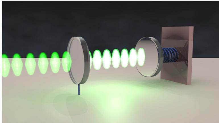
**Figure 1.** Three-dimensional representation of a standard optomechanical cavity with a spring mirror. Image courtesy of C Baker.
